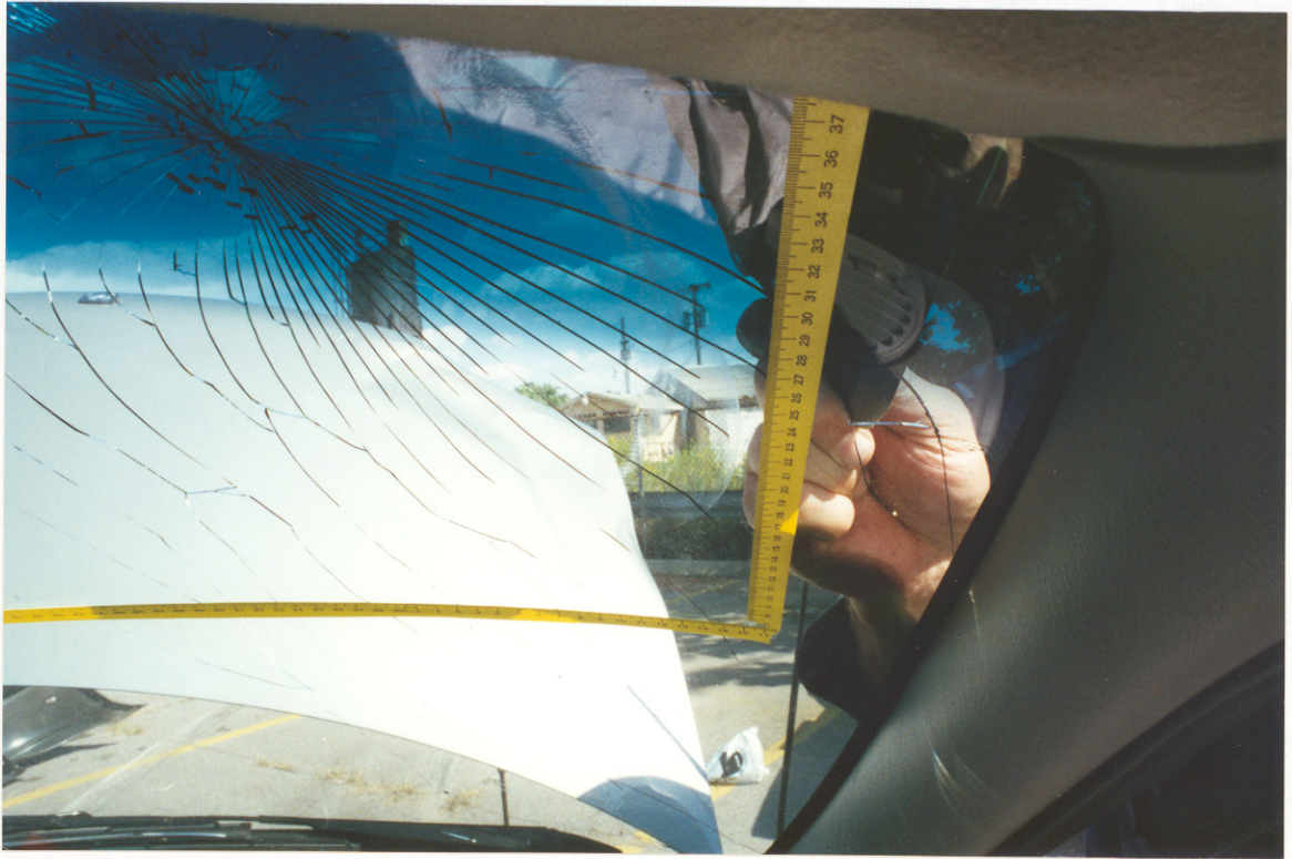
67. Close-up view of the windshield fracture and the air bag fabric transfers.
